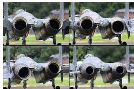
(b) Thrust Vectoring
